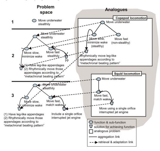
**Fig. 2.** Design trajectory of one of the projects that exemplify compound analogical design. Adapted from "Compound Analogical Design: Interaction Between Problem Decomposition and Analogical Transfer in Biologically Inspired Design," by S. Vattam, M. Helms, and A. Goel. *Proc. 3rd Int. Conf. Design Computing and Cognition*, pp. 377–396, 2008. Berlin: Springer. Copyright Springer 2008. Adapted with permission. [A color version of this figure can be viewed online at journals.cambridge.org/aie]
